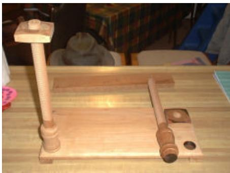
This photo shows how the spindles are mounted to the base of the sewing frame. Dry mounting the spindles allowed me to measure and mark where the slot went so the bindings would hang at the 90 from the work table of the sewing frame. I am not sure how this was done in period, but the “Try and Mark” method worked for me.
