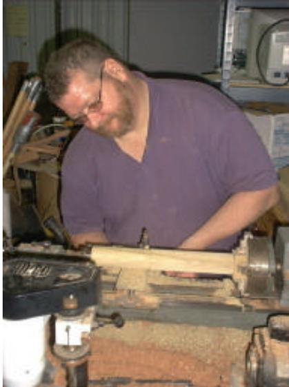
My hand and eye are not steady enough keep the spindles true to the tolerances using a wood lathe. I choose to cut the spindles on a small metal lathe to get the tolerances fine enough. I then used a free hand wood threading jig to make the threads on the screws.
