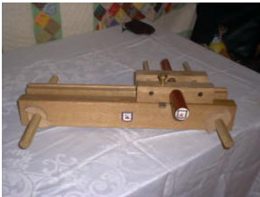
The photo on the left shows a Laying Press (or Cutting Press) and a Plough. In earlier periods the Laying Press was used with a draw knife to cut the ragged end of the bound book even. However, this produced ragged cuts and sometimes destroyed the work. Sometime in the 16<sup>th</sup> century the Plough was introduced. The introduction of the Plough called for a modification of the Laying Press. The plough allows for a more accurate cut due to the addition of the “rail”. It serves as a guide for
